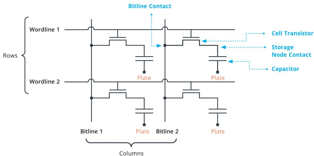
**FIGURE 1: FOUR DRAM CELLS IN A MEMORY ARRAY**
