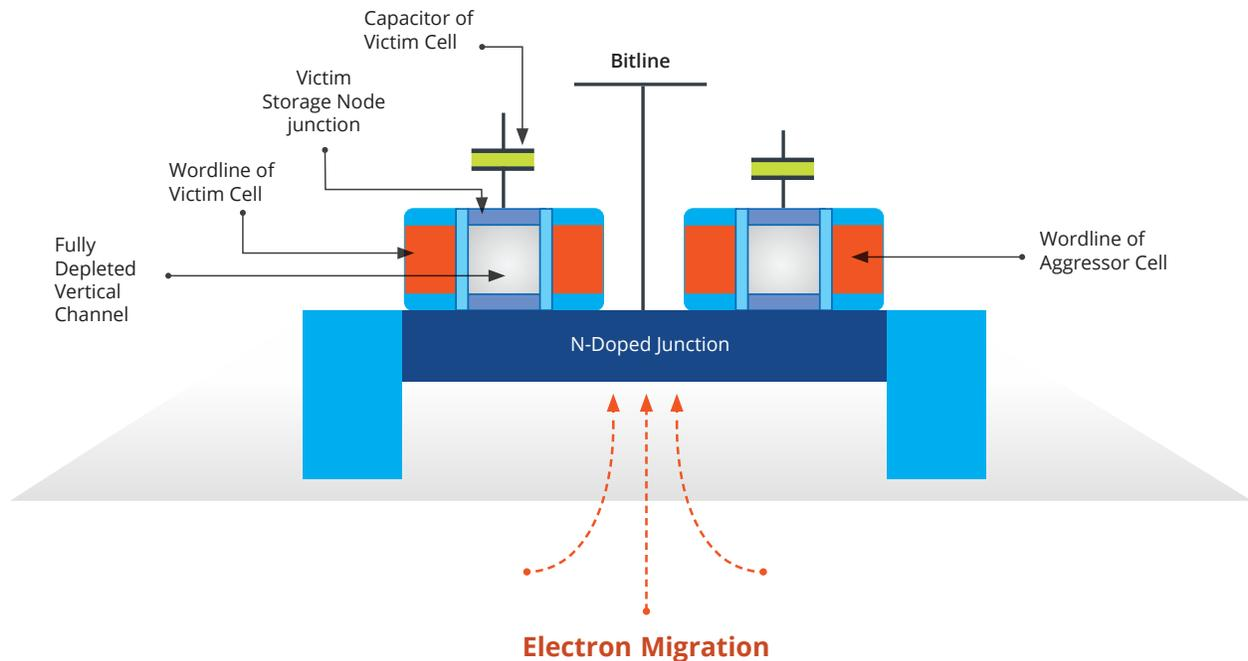
**FIGURE 4: CROSS SECTION OF TWO DRAM CELLS IN A MEMORY ARRAY USING SPIN MEMORY'S FULLY DEPLETED VERTICAL CHANNEL CELL TRANSISTORS. FULL DEPLETION ALLOWS THE CHANNEL TO BE ISOLATED FROM THE SUBSTRATE AND THEREFORE ISOLATES THE STORAGE NODE JUNCTIONS TOO.**
