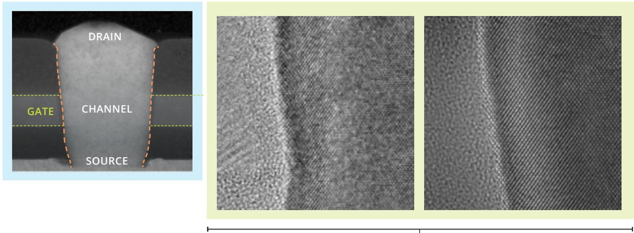
**Crystalline channel for high drive and low leakage**
