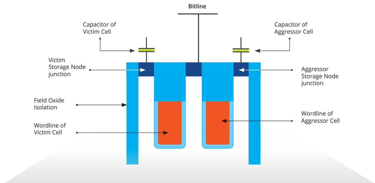
**FIGURE 2: CROSS SECTION OF TWO DRAM CELLS IN A MEMORY ARRAY WITH WORDLINE DIRECTION PERPENDICULAR TO PAGE AND BITLINE DIRECTION IN PLANE OF PAGE.**
